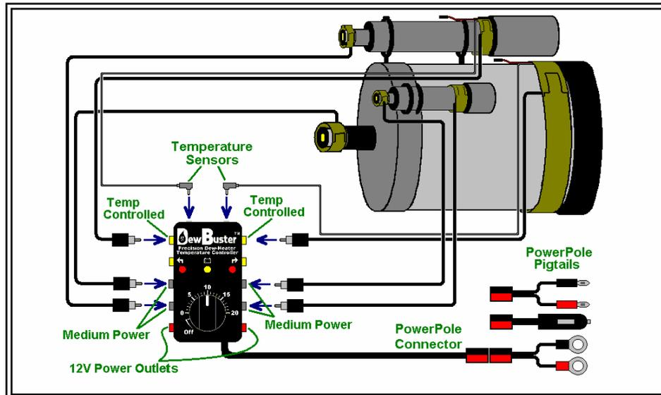
Medium Power Outputs (black) are intended for small heaters such as finderscope, eyepiece, Telrad, etc. that do not affect telescope performance so they are simply run at a higher power level than the Temperature Controlled Outputs to prevent dew without using a sensor. Medium Power normally runs at 40% power level but can be controlled manually as follows:
