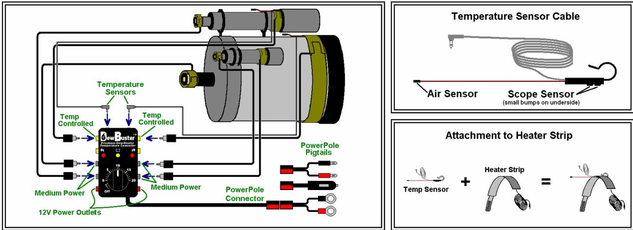
Color coded RCA Jacks on sides of controller are the Heater Outputs:
